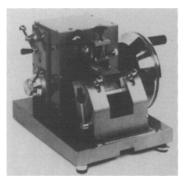
• Hacker Instruments is marketing its H/I-102 Precise Rotary Microtome. The instrument weighs 90 pounds and features a rapid advance control that remains permanently engaged and operates through a gear train free of springs. Advance is automatic to 40 microns in steps of one micron. Information: Hacker Instruments Inc., PO Box 657, Fairfield, NJ 07006.
