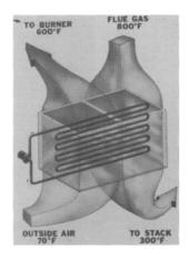
• Econo-Therm Systems has announced a preheat system which the firm says eliminates flue-gas condensation and consequent corrosion. The "Economic-Aire" system is a network of spiral-finned tubing looped through a twinchambered box, separated by an insulated steel wall with individual tubes welded into the divider. The heat-transfer fluid is moved by a centrifugal pump. Information: Econo-Therm Systems, 11321 K-Tel Dr., Minneapolis, MN 55343 (tele: 612-938-3100).
